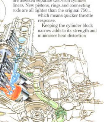
An oil-cooler and dual-rotor pump are included in the lubrication system, while the main engine coolant radiator is expanded by 25mm\* and uses a 10mm\* larger, thermostaticallycontrolled, electric fan.
